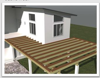
2. Use guideline text marked at 1¼" from each edge of tape to place Rot Shield on joists, with the text aligned to joist corners
