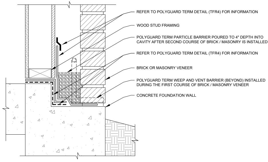
SECTION @ TERM © PARTICLE / TERMITE BARRIER IN MASONRY CAVITY WALL
