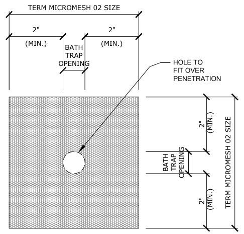
SECTION @ TERM<sup>©</sup> MICROMESH 02 WIRE SCREEN FOR ALL-PEST BATH TRAP
