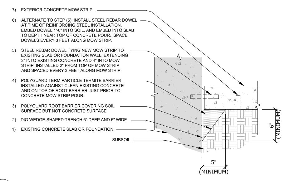
SECTION @ TERM® PARTICLE BARRIER UNDER MOW STRIP ADJACENT TO EXISTING CONCRETE STRUCTURE (BASED ON US ARMY CORPS OF ENGINEERS PACIFIC ISLAND INSTALLATION TERMITE BARRIER DETAIL)
