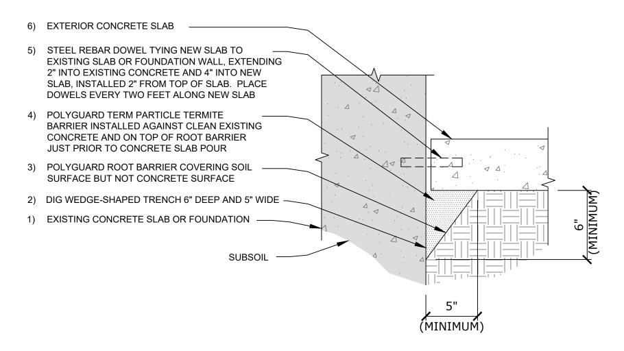
SECTION @ TERM<sup>©</sup> PARTICLE BARRIER UNDER CONCRETE SLAB (DRIVEWAY, PATIO, OR SLAB) ADJACENT TO EXISTING CONCRETE STRUCTURE
