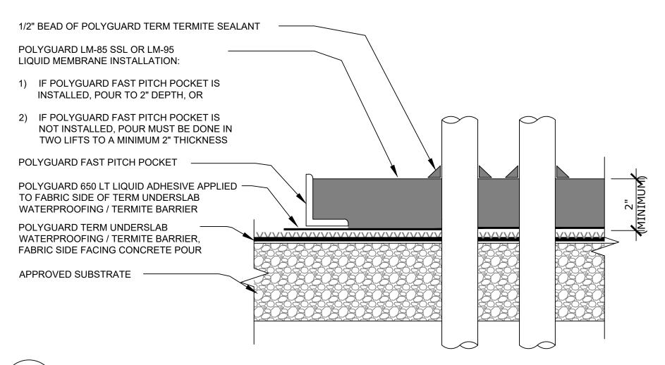
SECTION @ TERM<sup>©</sup> UNDERSLAB BARRIER PITCH POCKET WITH PENETRATIONS
