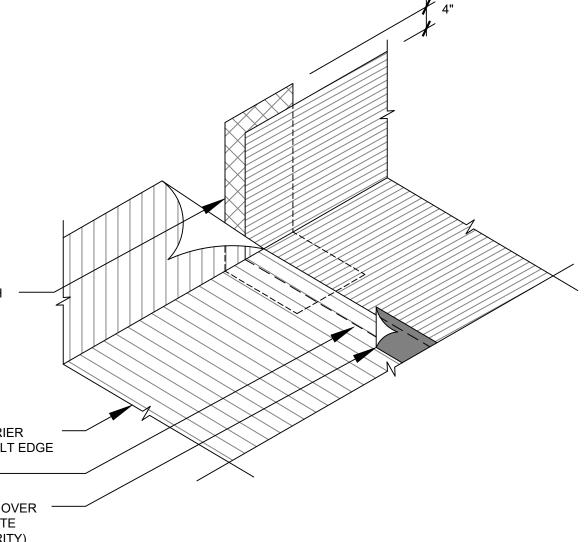
12" STRIP OF TERM FLASHING BARRIER APPLIED WITH ASPHALT SIDE UP TO RECEIVE TERM UNDERSLAB WATERPROOFING / TERMITE BARRIER BACKING, EXTEND FLASHING A MINIMUM 4" BEYOND TOP EDGE OF TERM UNDERSLAB WATERPROOFING / TERMITE BARRIER. ROLL FLAT WITH ROLLER.
