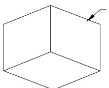
SIZE AN INSIDE CORNER BOOT FOR COVERAGE OF THE CORNER HEIGHT, AND PLACE IT INTO THE CORNER WITH THE POLYETHYLENE SIDE INTERFACING WITH THE CONCRETE FORM OR WALL
