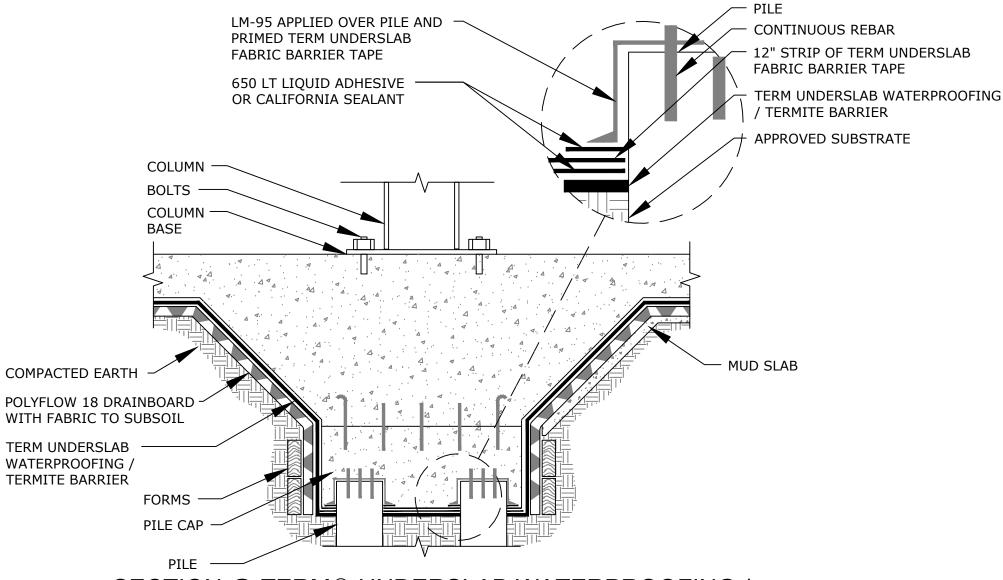
SECTION @ TERM® UNDERSLAB WATERPROOFING / TERMITE BARRIER GRADE BEAM PILE CAP (OPTION 1)
