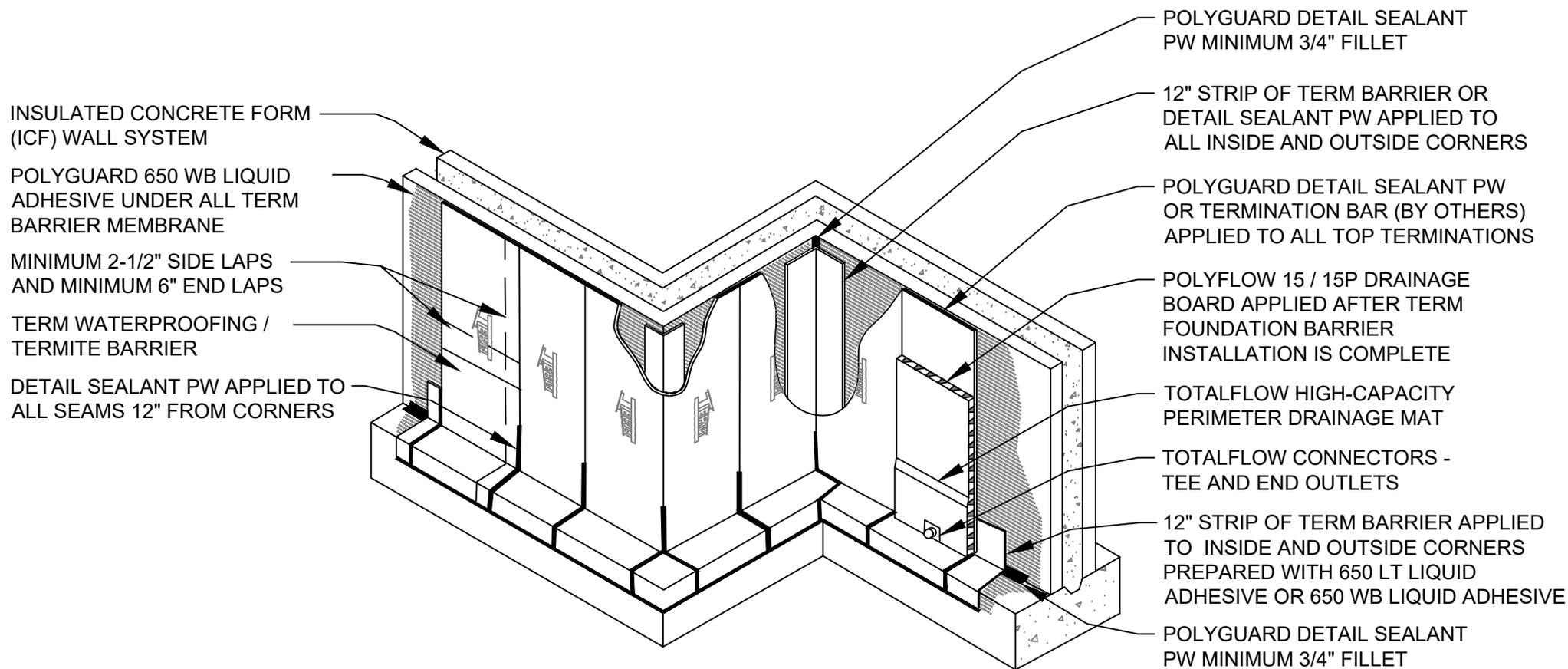
**TV1 ISOMETRIC @ TERM ICF WALL WATERPROOFING / TERMITE BARRIER APPLICATION**
