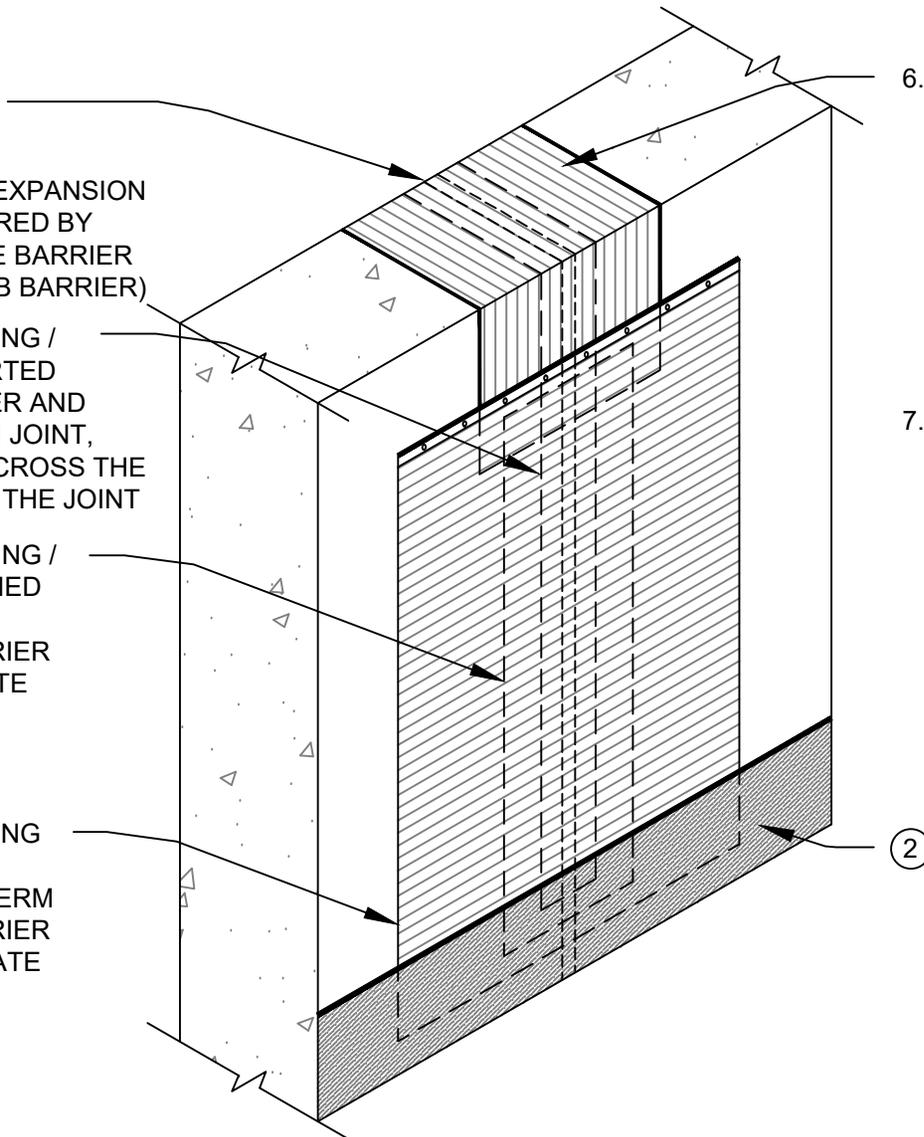
6. POLYGUARD ALUMAFASH - MINIMUM 4" WIDER THAN THE INVERTED 8" TERM WATERPROOFING / TERMITE BARRIER STRIP. PRIME THE SUBSTRATE(S) AS SHOWN IN STEP 4. INSTALL ALUMAFASH OVER ALL EXPOSED CONCRETE WHERE THE INVERTED STRIP IS INSTALLED. OVERLAP THE BELOW-GRADE TERM WATERPROOFING / TERMITE BARRIER IN A SHINGLE FASHION BY A MINIMUM 6"
