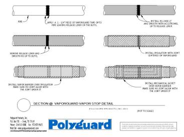
**Single layer insulation system (Chilled Water)** On Chilled Water application and sometimes on the high temperature side of cold service (25°F to 35°F) it is common to install a single layer of insulation with a factory applied vapor barrier.
