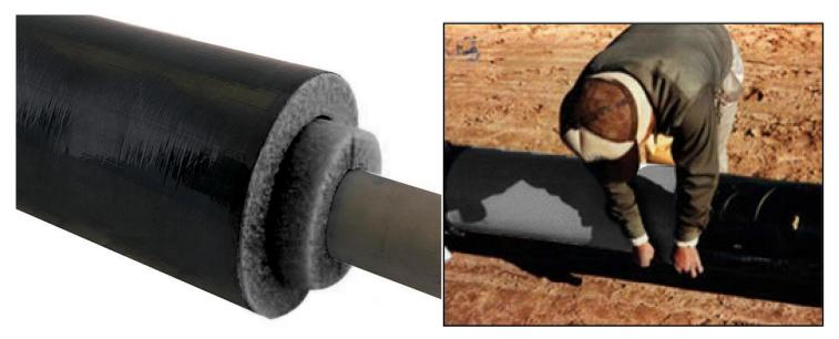
Install XPS single or double layered insulation as shown on pages 11 & 12. Install Polyguard I-50, No torch 125 and Insul-Shield over insulation depending on application. Thickness Tables: All Tables Calculated using 3EPlus v4.1. Table lists the greater thickness required to prevent condensation or limit heat gain to a maximum 8 BTU/hr/sq ft
